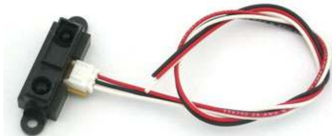
IR distance sensor w/cable (10cm-80cm) - GP2Y0A21YK0F
